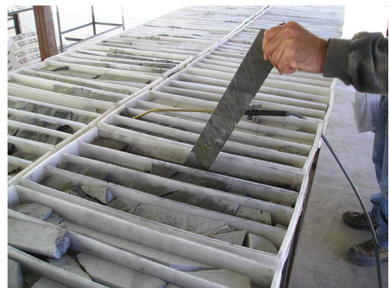
Orientation of core – note structures cutting across core
