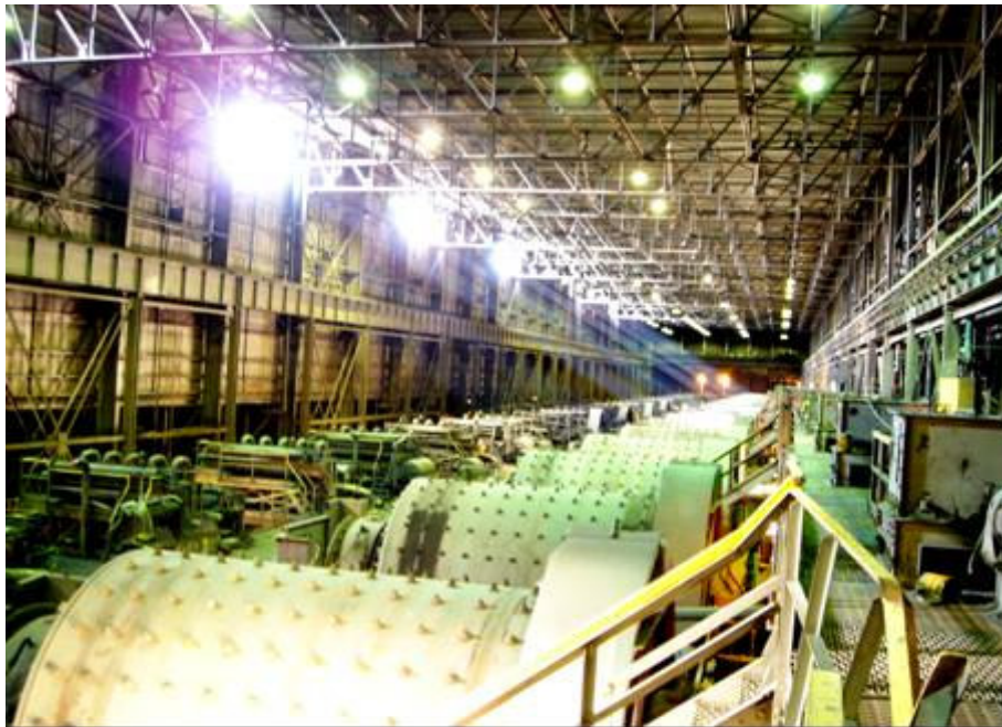
Figure 20-7 Concentrator interior showing some of the 33 rod mills owned by PolyMet
