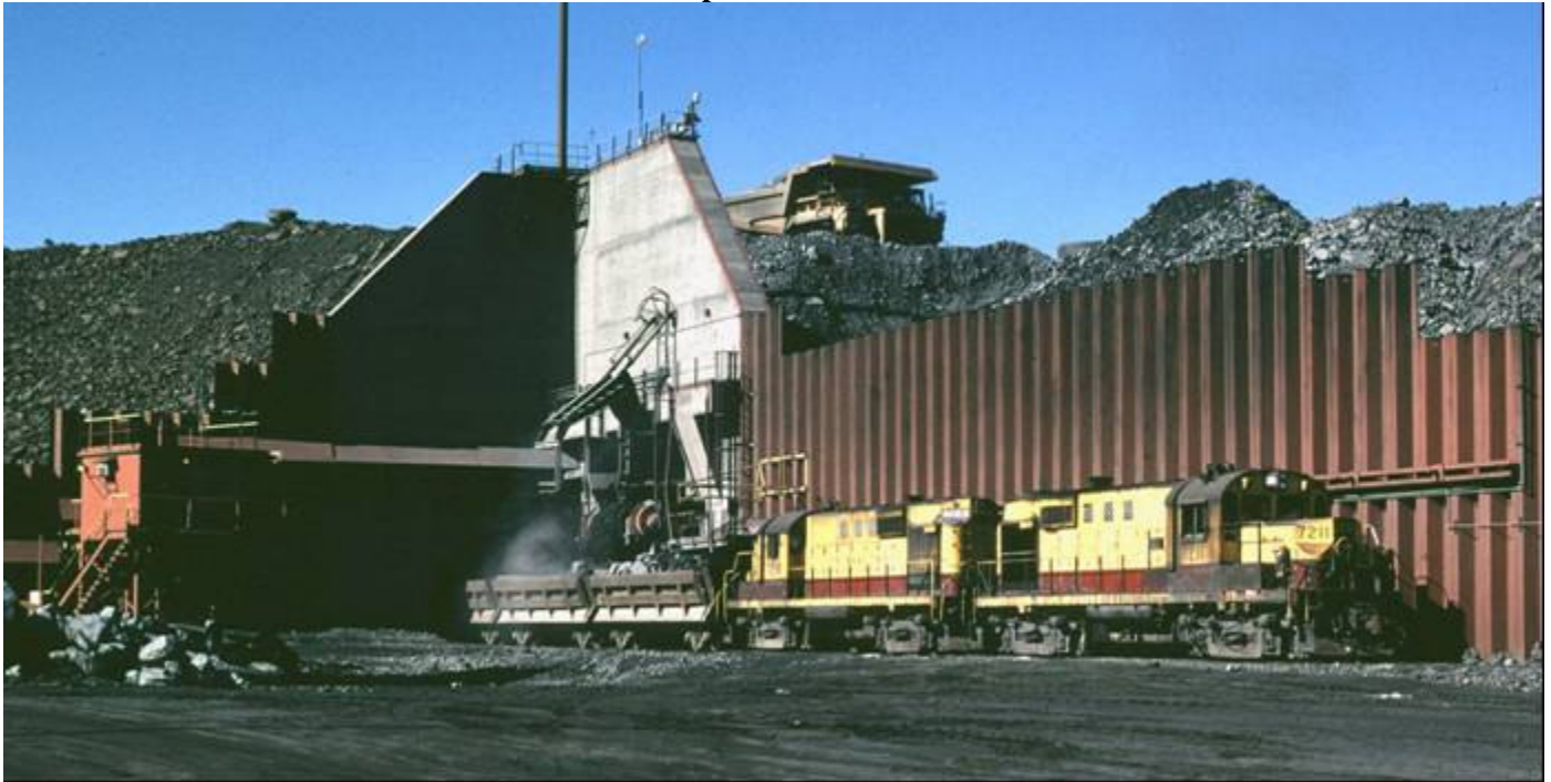
Figure 20-1 LTVSMC Rail Transfer Hopper in Operation
